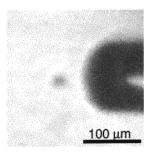
**Figure 6.** Microphotograph of photoelectrophoretic bead accumulation on a  $Mn_2O_3$ -coated n-type single-crystal silicon electrode. The accumulated 1  $\mu$ m beads appear as a dark spot next to the tip of the single mode optical fiber in the right half of the picture. Accumulation was performed by illuminating with 80  $\mu$ W for 1 min and scanning the applied potential between 0 and 0.6 V (200 mV/sec).
