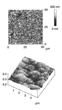
Figure 2. Tapping mode AFM images of a Mn<sub>2</sub>O<sub>3</sub> film deposited onto single crystal n-type silicon. The film thickness of this sample is approximately 270 nm with a medium roughness of 50 nm. (a) Lowresolution image showing the oriented granular structure of the Mn<sub>2</sub>O<sub>3</sub> film. Arrows indicate larger precipitates on the surface. (b) Highresolution surface plot of the same sample.
