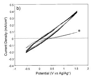
Figure 3. Current—voltage characteristics of  $Mn_2O_3$ -coated n-type silicon electrodes measured in 50 mM L-histidine solutions. The 10 consecutive cyclic voltammograms acquired in the dark (\*) and under illumination were measured (a) before and (b) after deposition of the streptavidin—agarose permeation layer. The scan rate was 100 mV/sec. (Electrochemical potentials were not compensated for ohmic potential drops across the low conductivity electrolyte.)
